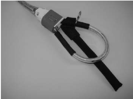
1 / Open the BRAIN Quick Release
