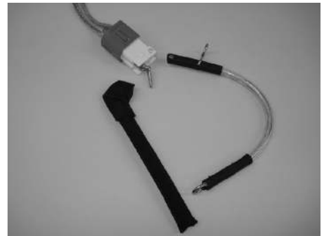
4 / Remove the locking tube from the depower loop
