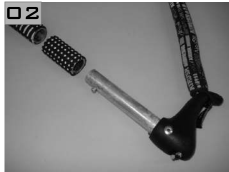
02 Add or remove the extension making sure to align the locator pin with the recess on the extension cover.
