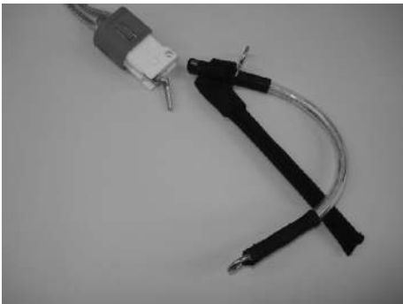
3 / Remove the depower loop
